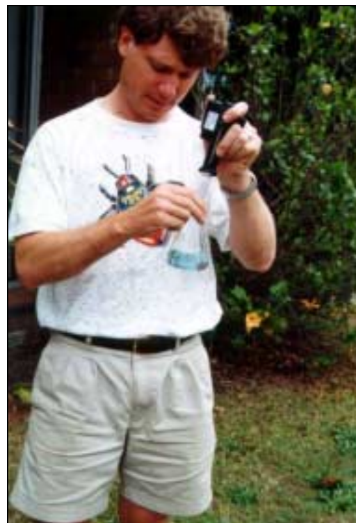
Plate 7. Taking field water quality measurements, water quality samples and doing an alkalinity titration test.
