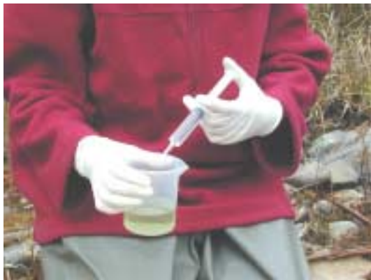
a) Before adding acid - water is green
