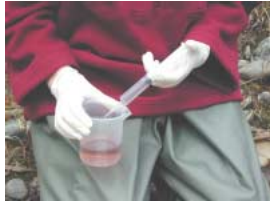
b) When titration reaches end point - water is pink
